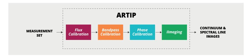
ARTIP operates on measurement sets and runs through several stages to generate continuum and spectral line images
